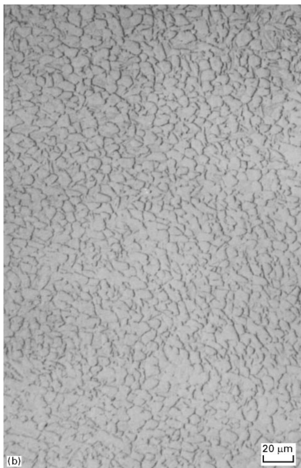
Figure 5 Effect of creep deformation at 760 °C for 20 h on the microstructure of Ti-25Al-10Nb-3V-1Mo (a) 760 °C/24 h/AC, (b) 1045 °C/0.5 h/FC + 760 °C/24 h/AC, and (c) 1200 °C/0.5 h/AC + 760 °C/45 h/AC.
