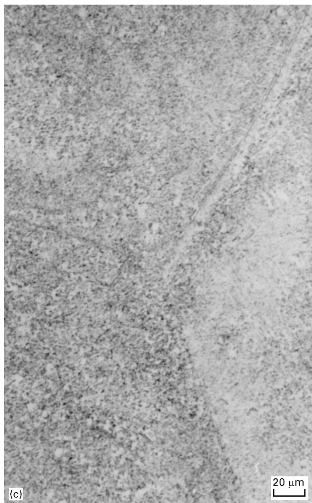
Figure 5 Effect of creep deformation at 760 °C for 20 h on the microstructure of Ti-25Al-10Nb-3V-1Mo (a) 760 °C/24 h/AC, (b) 1045 °C/0.5 h/FC + 760 °C/24 h/AC, and (c) 1200 °C/0.5 h/AC + 760 °C/45 h/AC.
