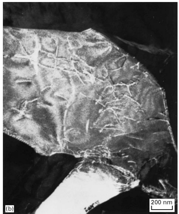
Figure 9 Dislocation substructures in Ti-24Al-11Nb annealed at 1200 °C/0.5 h/AC + 815 °C/8 h/AC and deformed under compressive creep conditions at 650 °C for 20 h (initial stress = 345 MPa); (a) bright-field image, and (b) weak-beam image.
