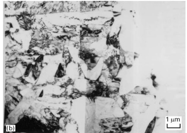
Figure 8 Bright-field transmission electron micrographs showing strain accommodation in the interdendritic \beta phase Ti-24Al-11Nb after creep deformation to 1.2% strain at 650 °C (initial stress = 345 MPa). (a) 1200 °C/0.5 h/AC + 815 °C/8 h/AC, and (b) 982 °C/4 h/AC.
